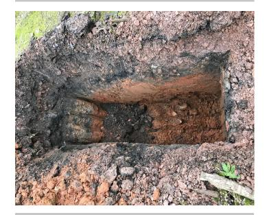
The ground investigation comprised of trial pitting with an excavator and the installation of ground gas and groundwater monitoring wells. A historic works building had been present on site for nearly 100 years and therefore the site was considered to have a high risk of contamination.
