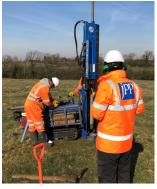
Although the site was agricultural fields at the time of the investigation, areas of deep made ground associated with the coal mining was identified and associated contamination testing associated with the former site usages was undertaken.
